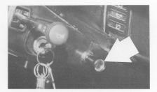
The first movement of the switch lever from the 'OFF' position brings on the side, tail, rear number plate and instrument lights. Further movement of the switch lever brings on the headlights also.
