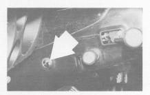
Air temperature can be varied by adjusting the position of the brass tap on the top left hand side of the engine just behind and to the right of the distributor. The maximum temperature is produced when the tap is parallel with the hose, and the temperature can be progressively reduced so that cold air is produced when the tap is perpendicular to the hose.
