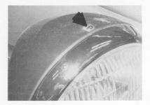
**Sidelights** – the light lens is removed by the two screws visible at the front of the lamps.
