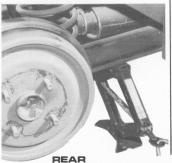
Whenever a wheel has been removed and replaced it is advisable to recheck the tightness of the wheel nuts after a further 1000 miles (1600 km).
