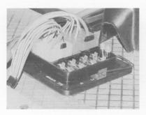
There are four cartridge-type fuses carried in a single block located under the bonnet in the centre of the flat area to the rear of the engine compartment.
