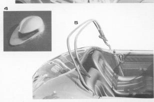
To fit tonneau cover, first locate on the two hooks on the rear bodywork then fasten along each side behind the doors; wind down windows, fasten front passenger side of the tonneau on two fasteners at base of windscreen, locate other side of tonneau over steering wheel, fasten centre zip and remaining fastener.
