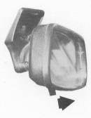
The rear-view mirror with antidazzle head is designed to break away from the windscreen on impact. To reduce mirror dazzle, pull the lever at the bottom of the mirror towards the rear of the car.
